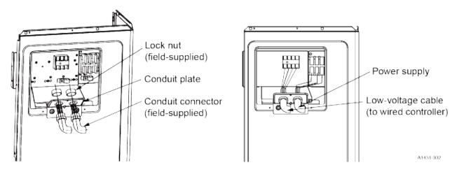
Figure 22: Connecting the power wiring from the disconnect switch into the control box for HH836E2S11 units - illustration 1
