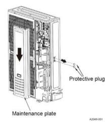
Figure 26: Connecting the power wiring from the disconnect switch into the control box for HH860E2S11 units - illustration 2
