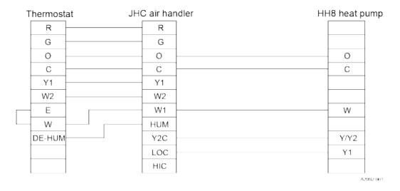
The Y1 input and Y/Y2 output on the outdoor unit must be wired as shown to the Y2C and LOC connections on the JHC air handling unit control board. The HUM input on the air handler control is for variable speed de-humidification operation.
