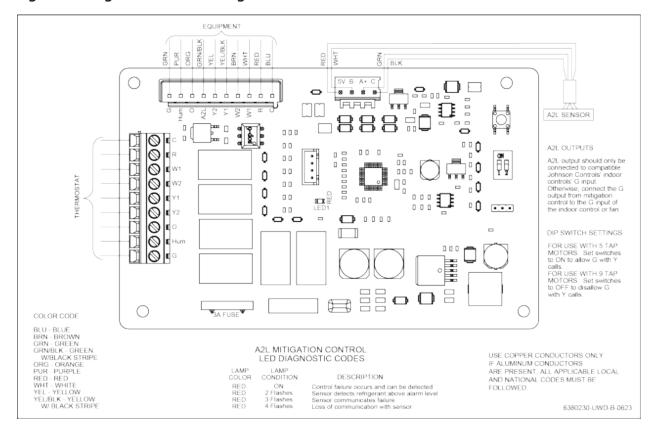
Figure 2 shows the DIP switches on the mitigation control board in the on position.
