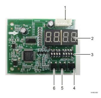
① **Note:** Figure 44 shows the 7-segment display control board with the black window control board cover removed.
