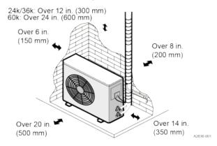
Figure 6: Alternative installation clearances for multiple units
