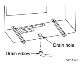
2. Connect the drain hose to the drain elbow.
