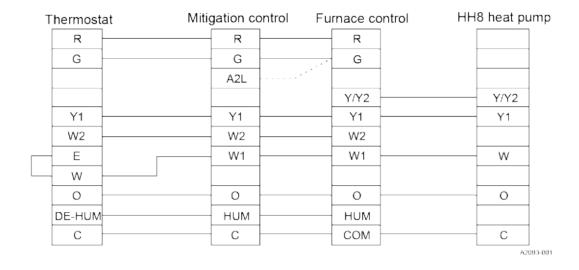
The mitigation control board has a bank of DIP switches. Both DIP switches must be in the 1 or on position. The room thermostat **must** control fossil fuel operation. W2 is applicable only on multi-stage gas furnace models. Use the mitigation control A2L output instead of the G output for Y82V, Z8VT, Y92V, Z9VT,Y9VV, and Z9VV gas furnace models. The HUM input on the furnace control is for variable speed de-humidification operation.
