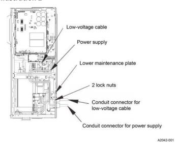
Figure 24: Connecting the power wiring from the disconnect switch into the control box for HH836E2S11 units - illustration 3
