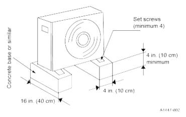
2. Install the anchor bolts into the base so they align with the anchoring position for the outdoor unit as shown in Figure 14 and Table 17.
