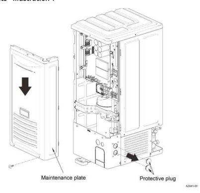
Figure 23: Connecting the power wiring from the disconnect switch into the control box for HH836E2S11 units - illustration 2
