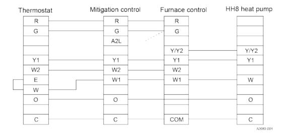
The mitigation control board has a bank of DIP switches. Both DIP switches must be in the 1 or on position. The room thermostat **must** control fossil fuel operation. W2 is applicable on only multi-stage gas furnace models. Use the mitigation control A2L output instead of the G output for Y81E, Z8ES, RL18, Y82E, Z8ET, Y91E, Z9ES, RG19, Y92E, and Z9ET gas furnace models.
