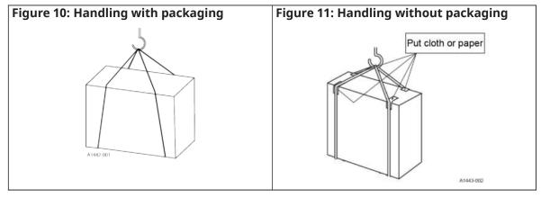
2. Ensure the unit is balanced and, if safe to do so, carefully lift up the unit.
