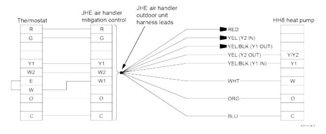
The mitigation control board has a bank of DIP switches. For use with a JHE air handler indoor model, both DIP switches must be in the 0 or off position.
