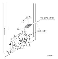
To braze the refrigerant lines and service valves, do the following:
