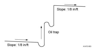
To install oil traps in the vapor line, do the following:
