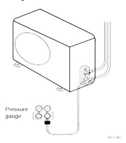
To check refrigerant system components, do the following:
