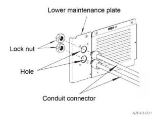
Figure 25: Connecting the power wiring from the disconnect switch into the control box for HH860E2S11 units - illustration 1
