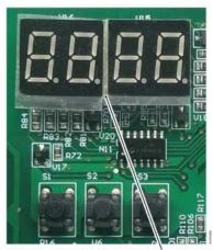
E displays with outdoor unit fault code or protection code, for example, E 13
