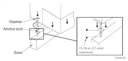
6. Check the length of the bolts. If the bolts are too long and could impede any future movement of the outdoor unit, cut them to a more appropriate length.
