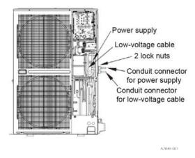
Figure 27: Connecting the power wiring from the disconnect switch into the control box for HH860E2S11 units - illustration 3
